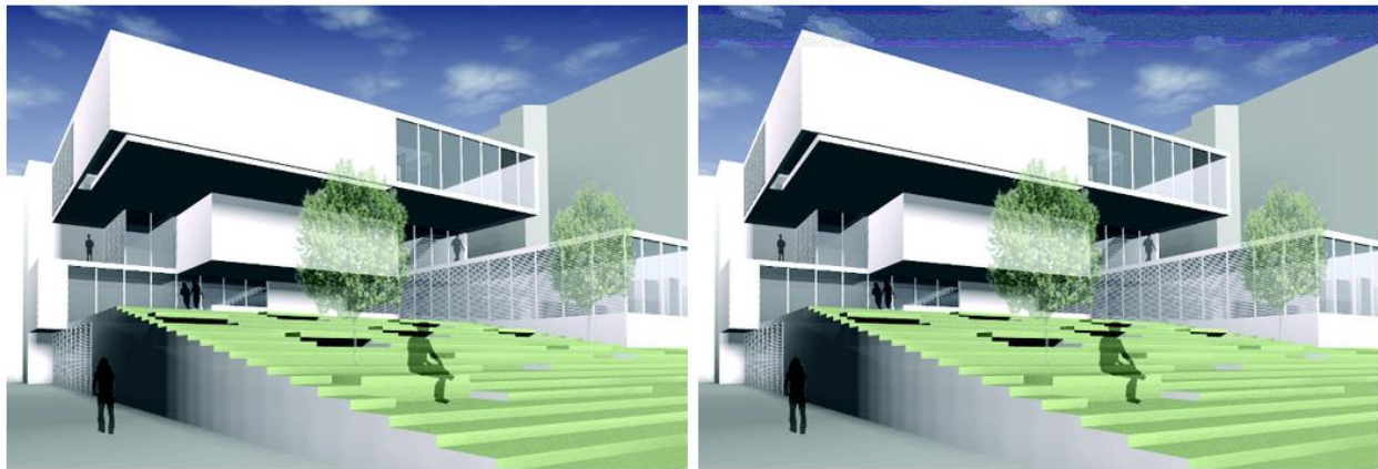
Figure 2. A Cover Image (left) and a Stego Image (right), side-by-side where the 5 least significant bits per byte are used to hide a secret image. Visible alterations can be observed at the top of the Stego Image.
