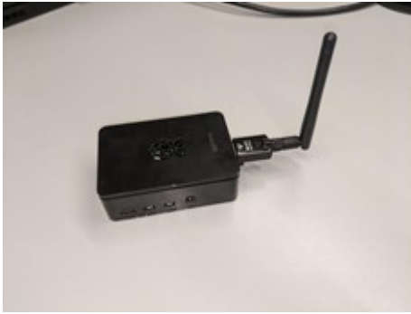
Fig. 1. Raspberry Pi 4 with WiFi Nation WN-H1 adapter
