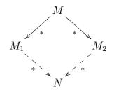
where the existence of the solid lines implies the existence of the dashed lines and the symbols \* indicate zero or more steps of reduction. Confluence of a TRS implies that every computation has at most one value. Note that not every TRS is confluent. A simple counterexample is the system
