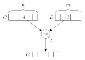
Figure 5.6. Naive implementation of resolution. The resolvent C' is computed by copying the literals from C except for  $\neg l$  and copying the literals from D except for l. n and m are the lengths of C and D. The time complexity is linear in n + m.
