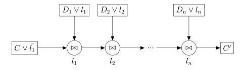
Figure 5.5. Conflict analysis — a linear sequence of resolutions. The  $\bowtie$  symbol represent the operation of resolution, and  $l_i$  are the pivot literals to be resolved out.  $C \vee \bar{l_1}$  is the initial input to conflict analysis (the *conflicting clause*).  $D_i \vee l_i$  clauses are clauses from the clause database. C' is the result of conflict analysis, called the *conflict clause*.
