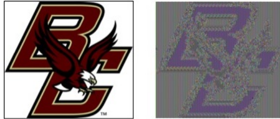
Figure 3: ECB encryption of a bit-mapped image. Large regions of the image with a single color lead to a large number of repeated blocks.
