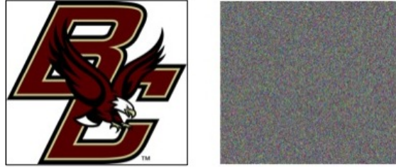
Figure 5: CBC encryption of a bit-mapped image. The chaining process alters the input to each encryption block, and the resulting ciphertext looks completely random.
